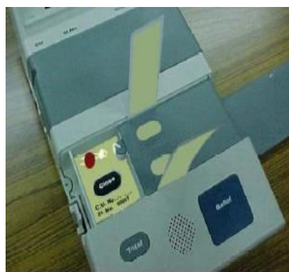
Sealing the inner door with Special Tag
