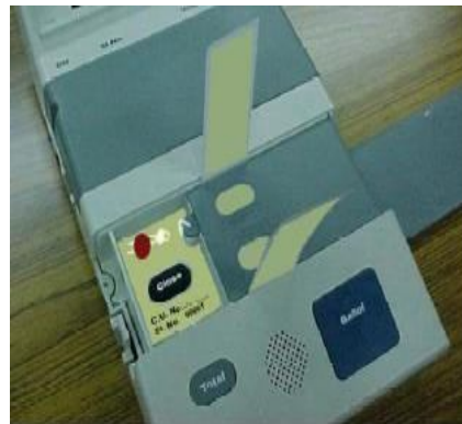
Sealing the inner door with Special Tag
